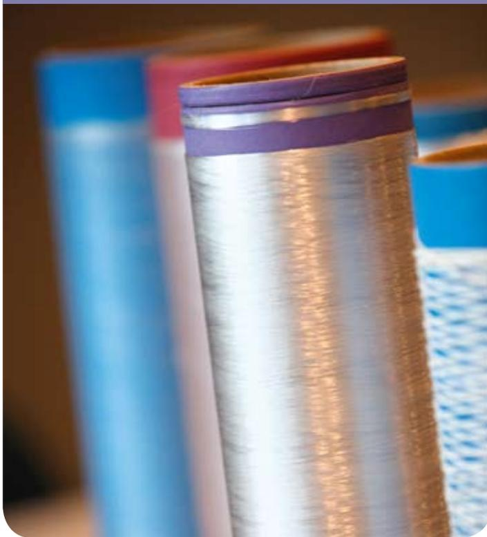
excellent for our experiments,” explains Ruys. “We built pilot extrusion lines that come close to the industrial process for them. Extrusion is obviously still not taking place optimally, in comparison with oil-based polymers. Nevertheless, we are already able to produce a small quantity of filaments.”
